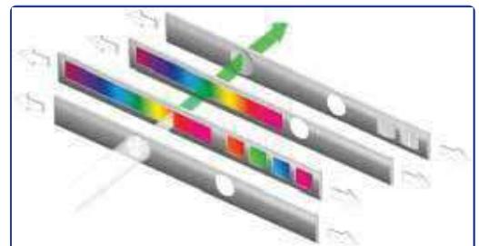
The ATL contains two LVF Monochromators, one for excitation and one for emission. In addition, a Linear Variable Dichroic mirror (340 - 740 nm) separates the two LVF Monochromators.
